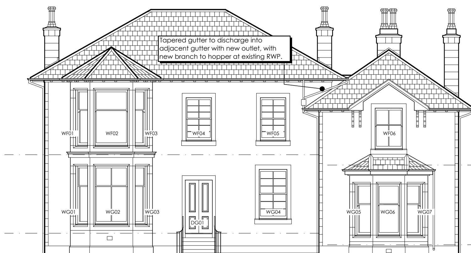
Front Elevation (SW) as Proposed Scale 1:100
