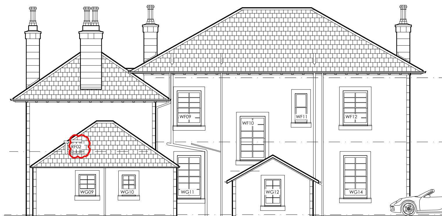
Rear Elevation (NE) as Proposed Scale 1:100
